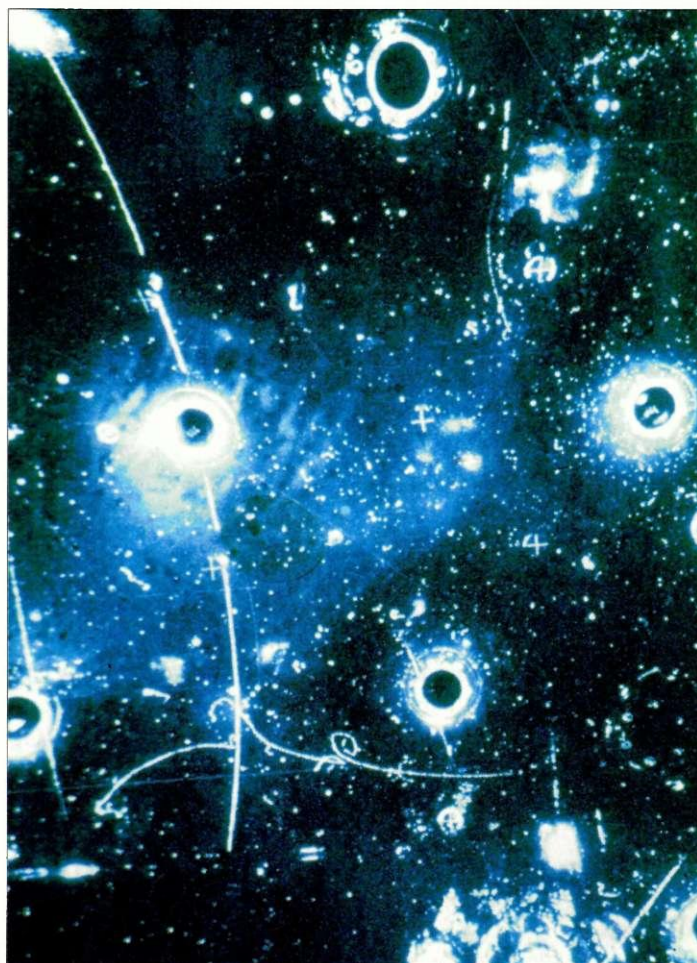
Neutral current – in 1973 the Gargamelle bubble chamber at CERN captured this historic photo showing how an invisible neutrino has jogged an electron.
