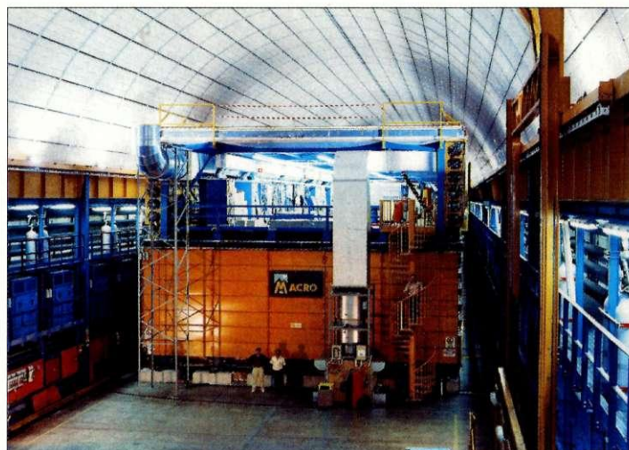
The MACRO detector in the Italian Gran Sasso underground laboratory. The lower, absorbing, half of the detector is interspersed with streamer tubes and is covered with scintillator and streamer chamber detectors (orange-coloured) to pick up muons emerging from reactions in the inner absorber. Additional information comes from the box-like "roof" of detectors above.
